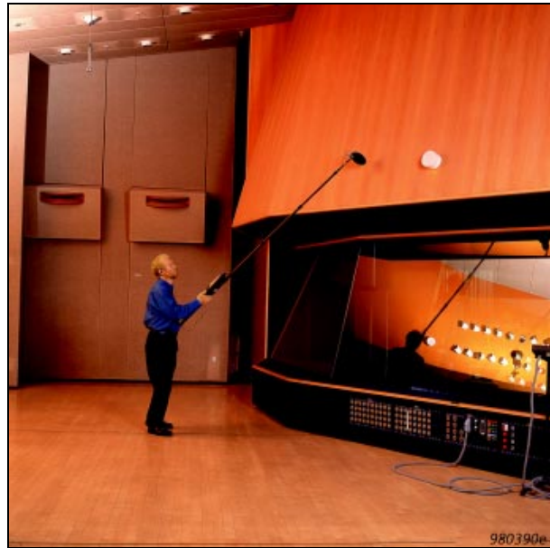
Fig. 7 Application example: Finding weak spots in sound insulation for a radio studio
